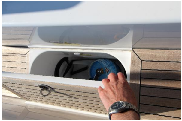
Deep Gas locker
