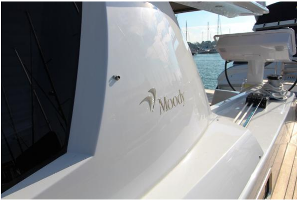
Control lines lead to the winches through guides
