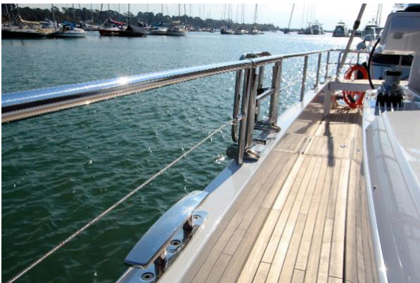
S/steel cleats in the up position
